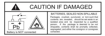
**NOTE:** These UPSs are shipped with the batteries disconnected. The batteries must be connected before putting these UPSs into service. Refer to Section 3 "Installation" for connecting the batteries.
